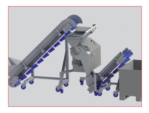
The high capacity **KUJ V** cube, strip and slice cutting machine can be integrated perfectly into a professional production line.
